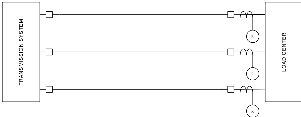
Figure 12 – Cohesive Load Center Remote to Transmission System
