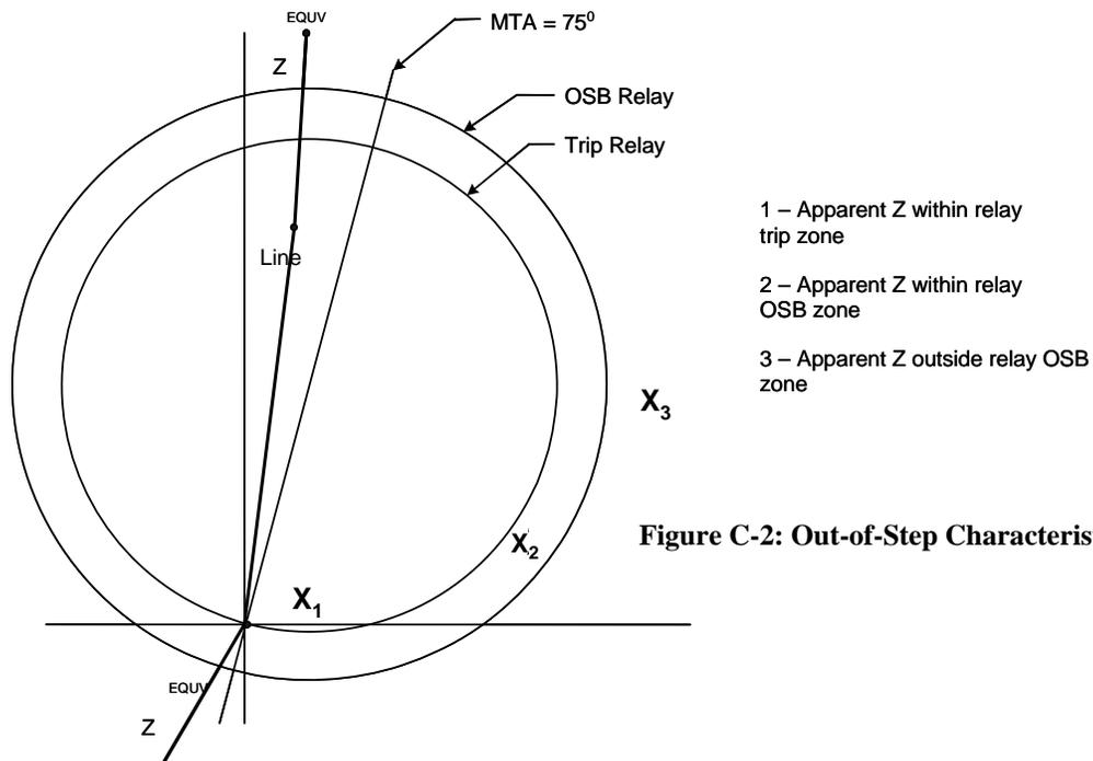
**Figure C-2: Out-of-Step Characteristics with Load**
