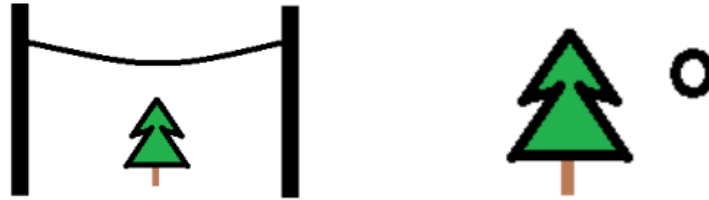
Figure 2: Vertical (Grow-in) and Horizontal (Blow-in) Conductor-to-Vegetation Gap Configurations
