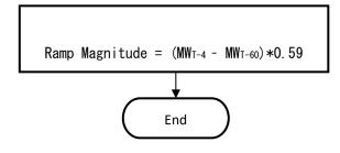
$(MW_{T-4} - MW_{T-60})$  represents the MW ramp of the generator resource/generator facility for a full minute prior to the event. The factor 0.59 adjusts this full minute ramp to represent the ramp that should have been achieved during the post-perturbation measurement period.
