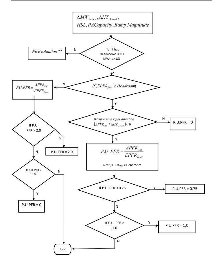
\*Check for adequate up headroom, low frequency events. Headroom must be greater than either 5MW or 2% of (HSL less PA Capacity), whichever is larger. If a unit does not have adequate up headroom, the unit is considered operating at full capacity and will not be evaluated for low frequency events.
