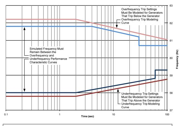
—— Generator Overfrequency Trip Modeling (Requirement R4 Parts 4.4-4.6)
