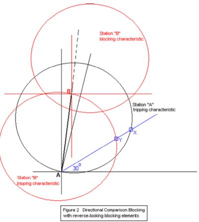
In Figure 2, blocking at Station "B" utilizes impedance elements which may or may not have offset. The settings of the blocking elements are traditionally based on external fault conditions only. It is unlikely that the blocking characteristic at Station "B" will extend into the load region of the tripping characteristic at Station "A". The loadability of Relay "A" will therefore almost invariably be determined by the impedance AX.
