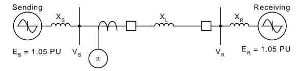
Figure 2 – Site-Specific Maximum Power Transfer Limit
