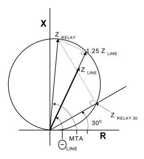
Figure 10 - Long Line relay Loadability
