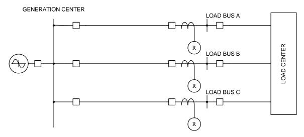
Figure 7 – Load Remote to Generation
