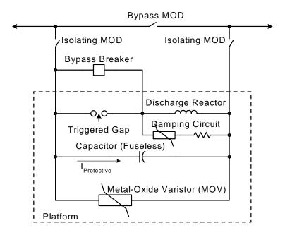
Figure 3 – Series Capacitor Components
