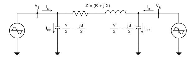
Lengthy transmission lines have significant series resistance, reactance, and shunt capacitance. The line resistance consumes real power when current flows through the line and increases the real power input during maximum power transfer. The shunt capacitance supplies reactive current, which impacts the sending end reactive power requirements of the transmission line during maximum power transfer. These line parameters should be used when calculating the maximum line power flow.
