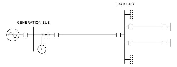
Figure 5 – Generation Remote to Load Center
