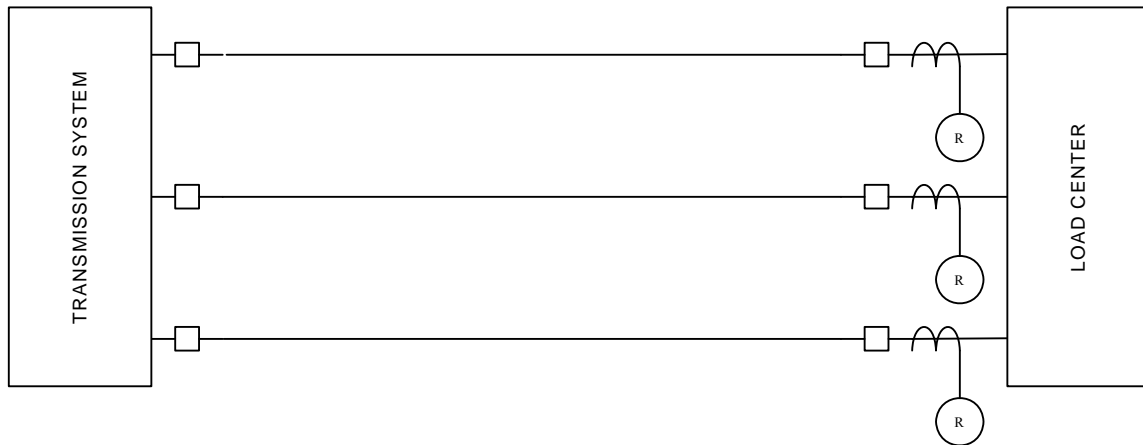
Figure 9 – Cohesive Load Center Remote to Transmission System
