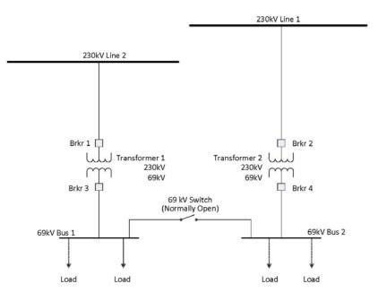
Figure 4 69 kV Networked Configuration with Normally Open Switch
