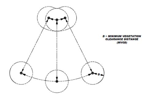
NERC indicated that conductor movements must be taken into account under FAC-003-2, and that the transmission owner is required to show that its approach to vegetation management under Requirement R3 will prevent encroachments under all expected line positions.<sup>64</sup> Thus, a transmission owner must manage vegetation to ensure it does not encroach into the MVCD under multiple conditions.
