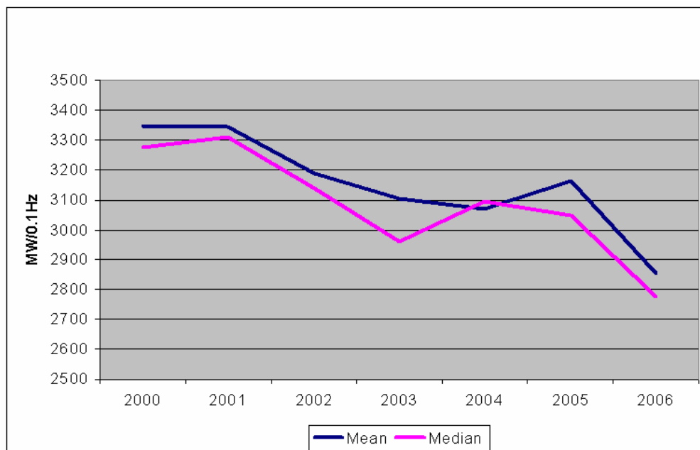
Figure 2 Updated Eastern Interconnection Frequency Response (NERC Resources Subcommittee)
