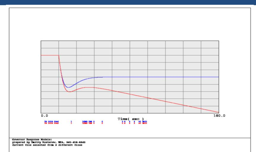
Blue = frequency response is sustained Red = generator has a "slow" load controller returning MW set-point
