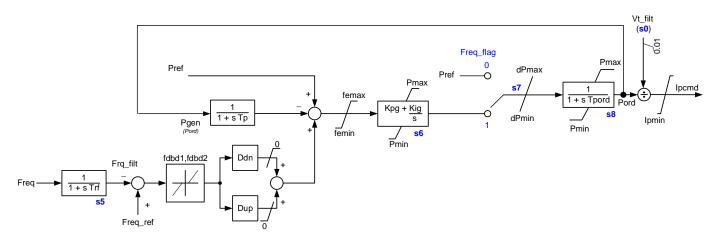
Figure 2: *DER\_A* Active Power-Frequency Controls
