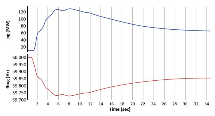
Figure 4.3: BESS Power vs. Frequency Performance
