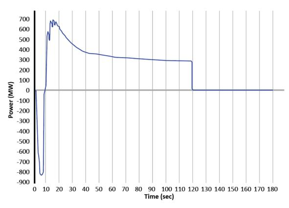
Figure 4.11: BESS Active Power Injection for Three Minutes
