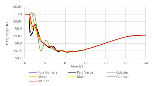
Figure 4.6: BESS Bus Frequencies for Five Small BESS
