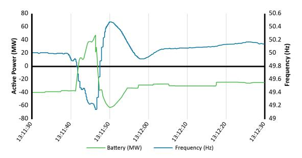
Figure 4.10: Hornsdale Battery Performance Due to the August 25, 2018, Event
