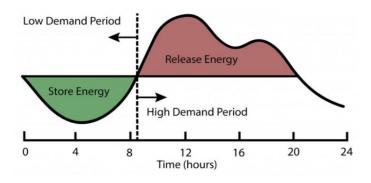
Figure I.5: Daily Energy Storage and Load Leveling<sup>7</sup>
