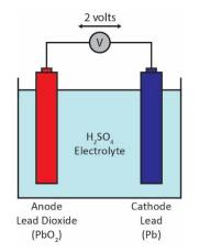
Figure I.1: Schematic of a Battery
