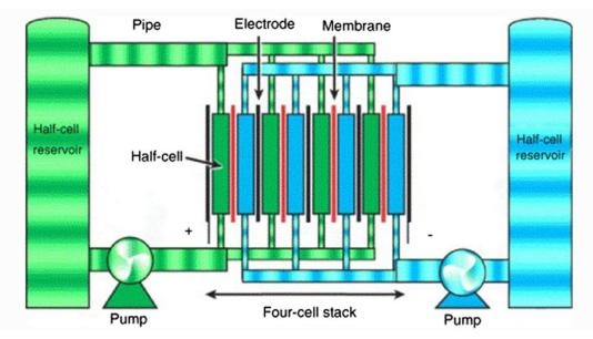
Figure 2.5: Schematic of Flow Batteries
