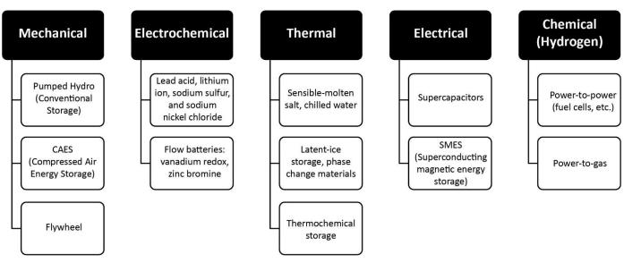
Figure 2.3: Classification of Storage Technologies<sup>21</sup>
