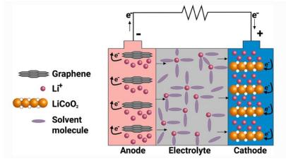
Figure 2.4: Ion flow in lithium-Ion battery<sup>22</sup>
