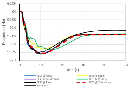
Figure 4.9: Grid Median Frequency Comparison
