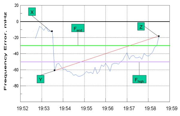
**Figure 27**. Plot of a recovery following a contingency, showing some significant points and parameters considered by the Processing phase program for this event.
