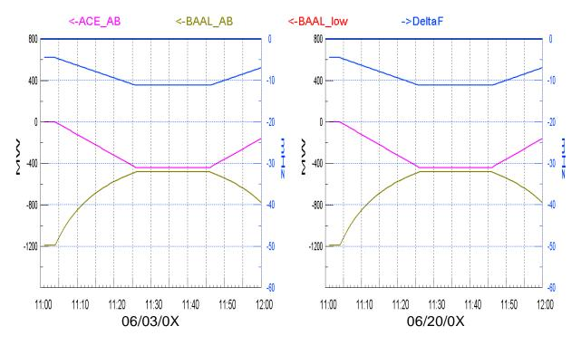
**Figure 14.** Combined ACE trend of the two BAs in Figure 13 when compared with the  $BAAL_{low}$  for the aggregating BA.
