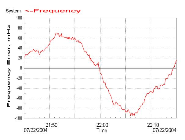
**Figure 16**. Plot of frequency during a recent frequency excursion lacking a signature of a large contingency.
