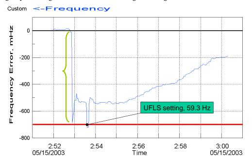
**Figure 5**. ERCOT frequency response to a large event. The bracket indicates the magnitude of the frequency drop considered for the estimate of P-Frequency-Response. The second event, occurring between 2:53 and 2:54, is not considered for calculation of P-Frequency-Response as frequency deviation resulting from it is influenced by UFLS shedding a large magnitude of load.
