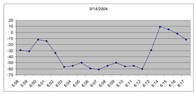
**Figure 15**. Plot of frequency during a recent frequency excursion lacking a signature of a large contingency.
