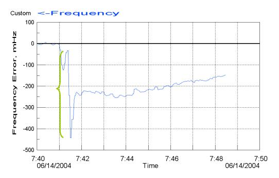
**Figure 3**. WECC frequency response to a large event. The bracket indicates the magnitude of the frequency drop considered for the estimate of P-Frequency-Response.
