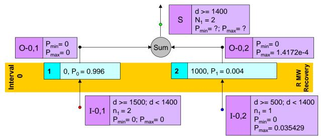
**Figure 21**. Finding *P*<sub>min</sub> and *P*<sub>max</sub>.
