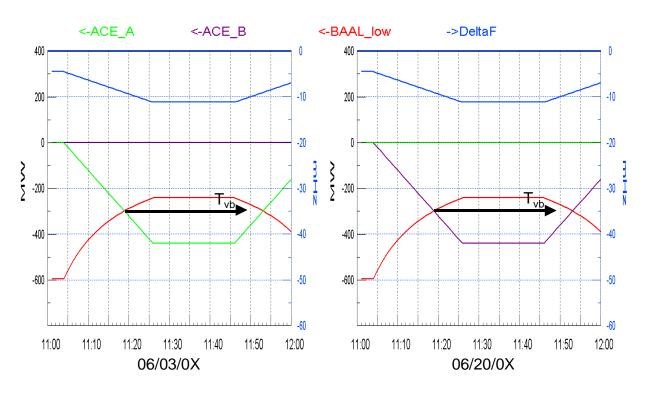
**Figure 13**. ACE trends of two BAs in two different one-hour periods when separately compared with each BA's BAAL<sub>low</sub>.
