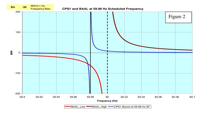
The Balancing Authority ACE Limit ("BAAL") was developed "from the ground up", considering the targeted research and development of Interconnection-specific Frequency Relay Limits, Frequency Abnormal Limits, and Frequency Trigger Limits. As the BAAL calculation is not a function of the Scheduled Frequency, its associated curves do not shift in a manner similar to CPS1, rather the limits remain symmetric about 60 Hz. as illustrated in Figures 1 and 2.
