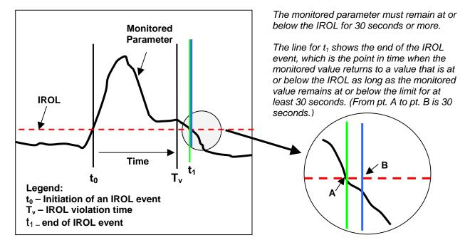
The following example is shown in the chart below. The IROL that has been exceeded has a  $T_v$  of 10 minutes. The monitored value exceeds the IROL for 15 minutes, then the monitored value returns to a value that is below that IROL for just 20 seconds, then the monitored value exceeds the IROL for another 10 minutes – then the monitored value returns to a value that is below the IROL for 2 hours. The duration of the event that must be reported is:
