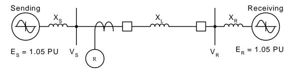
Figure 2: Site-Specific Maximum Power Transfer Limit
