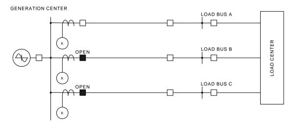
Figure 6 – Generation Connected to System – Multiple Lines
