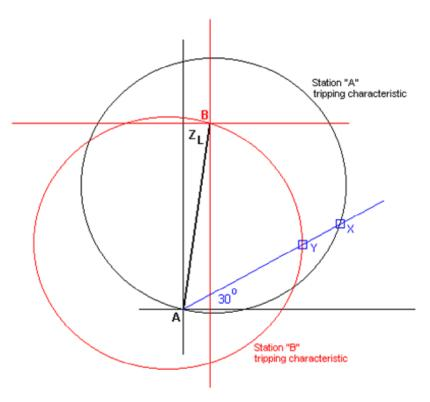
Figure B-1: Permissive Overreaching Transferred Trip (unmodified)
