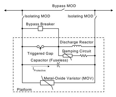
**Figure 3: Series Capacitor Components**
