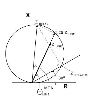
Figure 10 – Long Line relay Loadability
