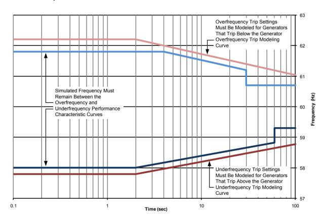
Generator Overfrequency Trip Modeling (Requirement R4 Parts 4.4-4.6) Overfrequency Performance Characteristic (Requirement R3 Part 3.2) Underfrequency Performance Characteristic (Requirement R3 Part 3.1) Generator Underfrequency Trip Modeling (Requirement R4 Parts 4.1-4.3)
