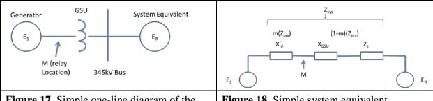
**Figure 17.** Simple one-line diagram of the system to be evaluated.
