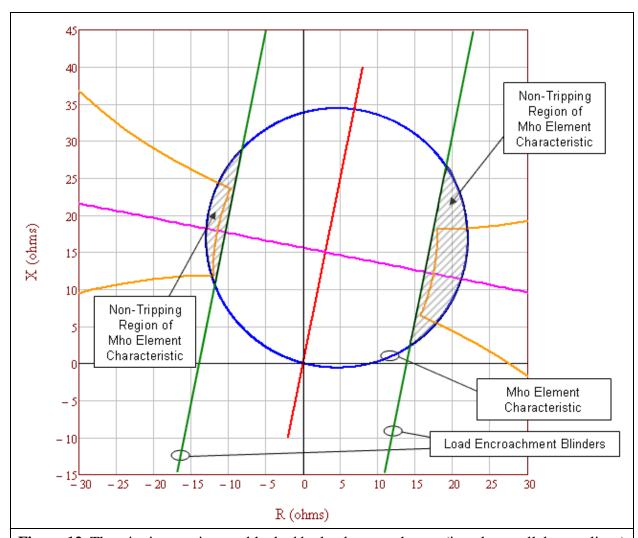
**Figure 12.** The tripping portion not blocked by load encroachment (i.e., the parallel green lines) of the mho element characteristic (i.e., the blue circle) is completely contained within the unstable power swing region (i.e., the orange characteristic). Therefore, the mho element characteristic meets the PRC-026-1 – Attachment B, Criteria A.
