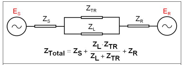
**Figure 6.** Reduced two bus system with sending-end source impedance  $Z_S$ , receiving-end source impedance  $Z_R$ , line impedance  $Z_L$ , and transfer impedance  $Z_{TR}$ .
