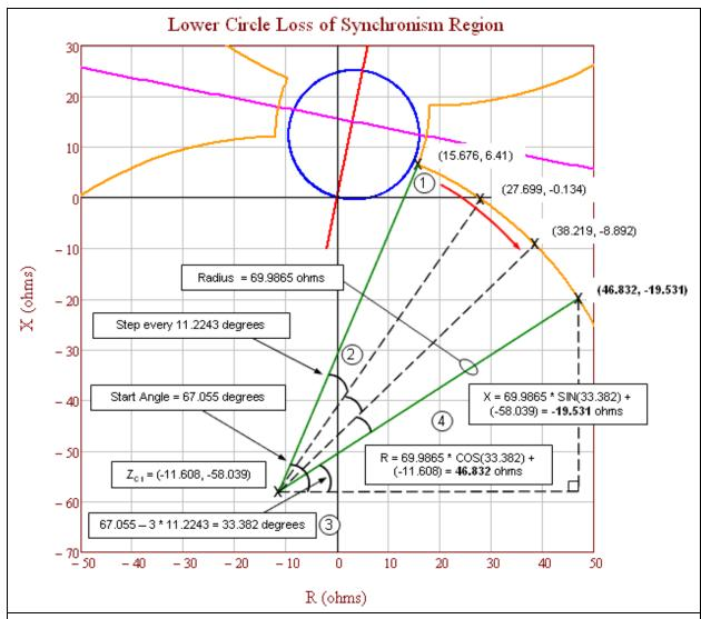
**Figure 15d:** Lower circle loss of synchronism region showing the final steps to calculate the coordinates of the points on the circle. 1) Start at the intersection with the lens shape and proceed in a clockwise direction. 2) Advance the step angle for each point. 3) Calculate the new angle after step advancement. 4) Calculate the R–X coordinates.
