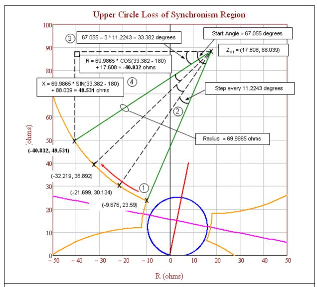
**Figure 15h:** Upper circle loss of synchronism region showing the final steps to calculate the coordinates of the points on the circle. 1) Start at the intersection with the lens shape and proceed in a clockwise direction. 2) Advance the step angle for each point. 3) Calculate the new angle after step advancement. 4) Calculate the R-X coordinates.
