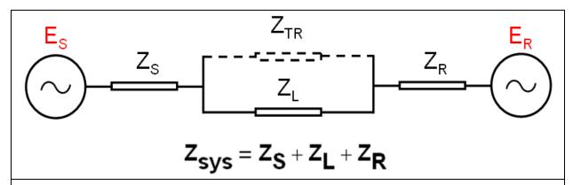
**Figure 7.** Reduced two bus system with sending-end source impedance  $Z_S$ , receiving-end source impedance  $Z_R$ , line impedance  $Z_L$ , and transfer impedance  $Z_{TR}$  removed.
