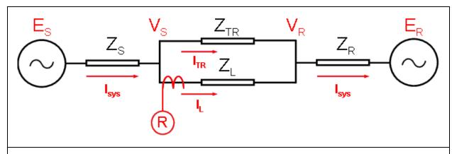
Figure 3. System impedance as seen by relay R.
