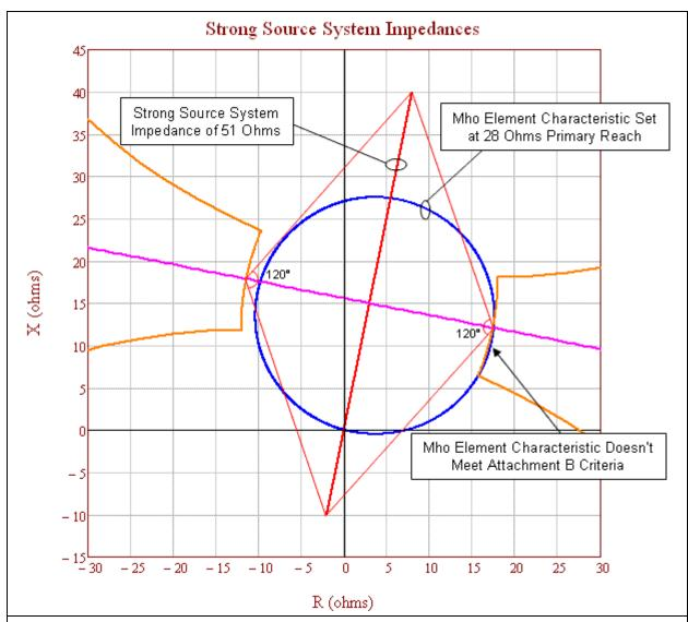
**Figure 8.** A strong-source system with a line impedance of  $Z_L = 20.4$  ohms (i.e., the thicker red line). This mho element characteristic (i.e., the blue circle) does not meet the PRC-026-1 – Attachment B, Criteria A because it is not completely contained within the unstable power swing region (i.e., the orange characteristic).
