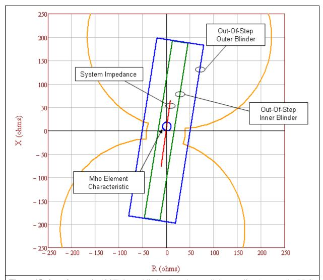
**Figure 15.** Out-of-step trip (OST) inner blinder (i.e., the parallel green lines) meets the PRC-026-1 – Attachment B, Criteria A because the inner OST blinder initiates tripping either On-The-Way-In or On-The-Way-Out. Since the inner blinder is completely contained within the unstable power swing region (i.e., the orange characteristic), it meets the PRC-026-1 – Attachment B, Criteria A.
