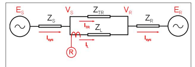
**Figure 13:** The infeed diagram shows the impedance in front of the relay R with the parallel transfer impedance included. As the parallel transfer impedance approaches infinity, the impedances seen by the relay R in the forward direction becomes  $Z_L + Z_R$ .
