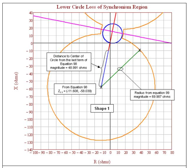
**Figure 15a:** Lower circle loss of synchronism region showing the coordinates of the circle center and the circle radius.
