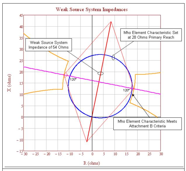
**Figure 9.** A weak-source system with a line impedance of  $Z_L = 20.4$  ohms (i.e., the thicker red line). This mho element characteristic (i.e., the blue circle) meets the PRC-026-1 – Attachment B, Criteria A because it is completely contained within the unstable power swing region (i.e., the orange characteristic).
