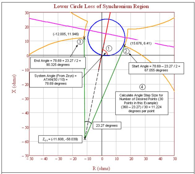
**Figure 15c:** Lower circle loss of synchronism region showing the steps to calculate the start angle, end angle, and the angle step size for the desired number of calculated points. 1) Calculate the system angle. 2) Calculate the start angle. 3) Calculate the end angle. 4) Calculate the angle step size for the desired number of points.
