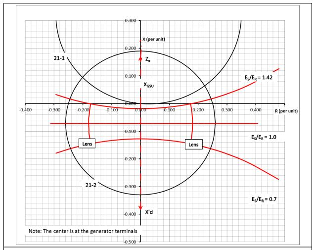
Figure 19. Swing impedance graph for impedance relays at a generating facility.
