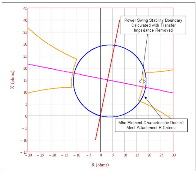
**Figure 10.** This is an example of an unstable power swing region (i.e., the orange characteristic) with the transfer impedance removed. This relay mho element characteristic (i.e., the blue circle) does not meet PRC-026-1 – Attachment B, Criteria A because it is not completely contained within the unstable power swing region.
