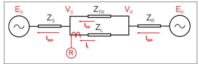
**Figure 14:** The infeed diagram shows the impedance behind relay R with the parallel transfer impedance included. As the parallel transfer impedance approaches infinity, the impedances seen by the relay R in the reverse direction becomes  $Z_S$ .
