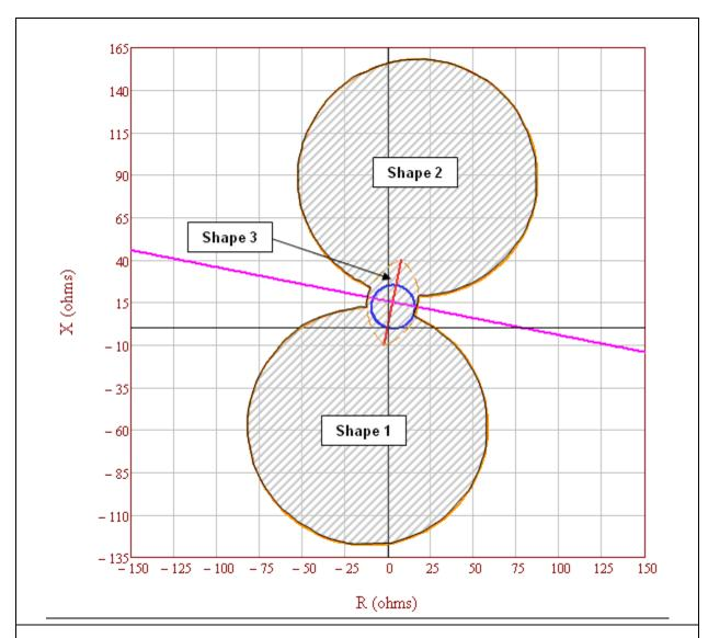
**Figure 2.** Full graphic of unstable power swing region formed by the union of three shapes in the impedance (R-X) plane: Shape 1) Lower loss of synchronism circle, Shape 2) Upper loss of synchronism circle, and Shape 3) Lens. The mho element characteristic is completely contained within the unstable power swing region, therefore it meets PRC-26-1 – Attachment B, Criteria A, No.1.
