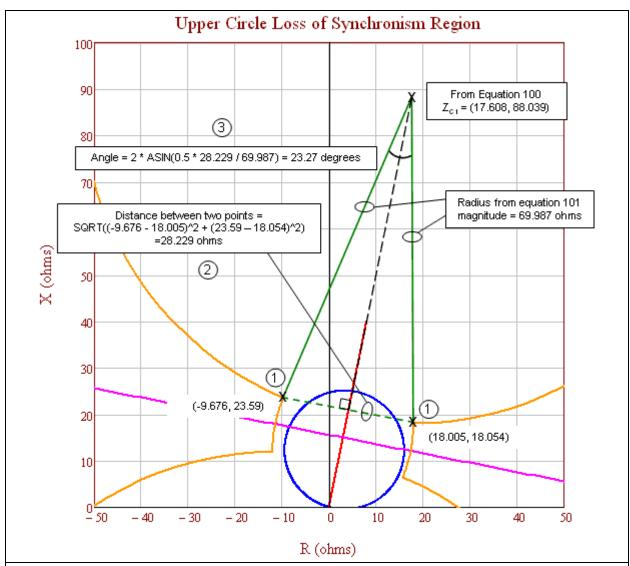
**Figure 15f:** Upper circle loss of synchronism region showing the first steps to calculate the coordinates of the points on the circle. 1) Identify the upper circle points that intersect the lens shape where the sending-end to receiving-end voltage ratio is 1.43 (see lens shape calculations in Tables 2-7). 2) Calculate the distance between the two upper circle points identified in Step 1. 3) Calculate the angle of arc that connects the two upper circle points identified in Step 1.
