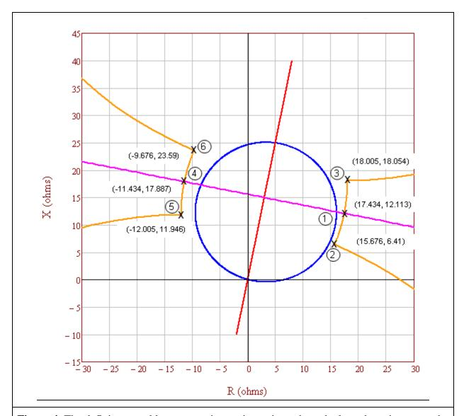
**Figure 4.** The defining unstable power swing region points where the lens shape intersects the lower and upper loss of synchronism circle shapes and where the lens intersects the equal EMF (electromotive force) power swing.
