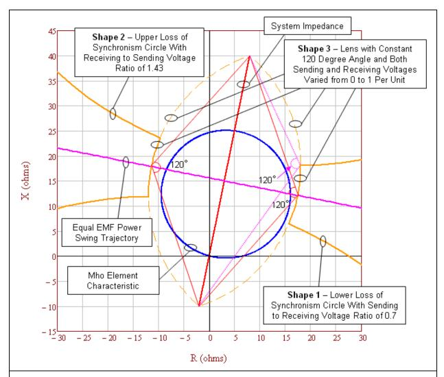
**Figure 1.** An enlarged graphic illustrating the unstable power swing region formed by the union of three shapes in the impedance (R-X) plane: Shape 1) Lower loss of synchronism circle, Shape 2) Upper loss of synchronism circle, and Shape 3) Lens. The mho element characteristic is completely contained within the unstable power swing region (e.g., it does not intersect any portion of the unstable power swing region), therefore it complies with PRC-026-1 – Attachment B. Criteria A, No. 1.
