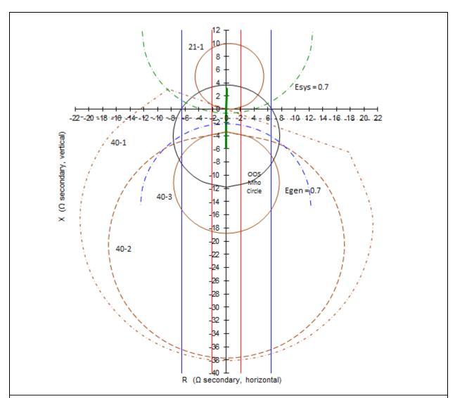
**Figure 22:** Double Blinder Out-of-Step Scheme with unit impedance data and load-responsive protective relay impedance characteristics for the example 940 MVA generator, scaled in relay secondary ohms.
