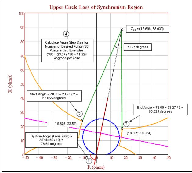
**Figure 15g:** Upper circle loss of synchronism region showing the steps to calculate the start angle, end angle, and the angle step size for the desired number of calculated points. 1) Calculate the system angle. 2) Calculate the start angle. 3) Calculate the end angle. 4) Calculate the angle step size for the desired number of points.
