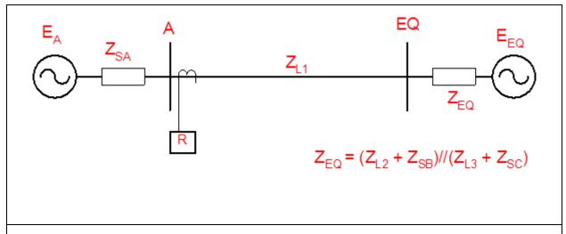
**Figure 15k.** Three-terminal line reduced to a two-terminal line.
