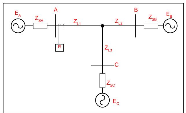
**Figure 15j.** Three-terminal line. To evaluate the load-responsive protective relays on the three-terminal line at Terminal A, the circuit in Figure 15j is first reduced to the equivalent circuit shown in Figure 15k. The evaluation process for the load-responsive protective relays on the line at Terminal A will now be the same as that of the two-terminal line.
