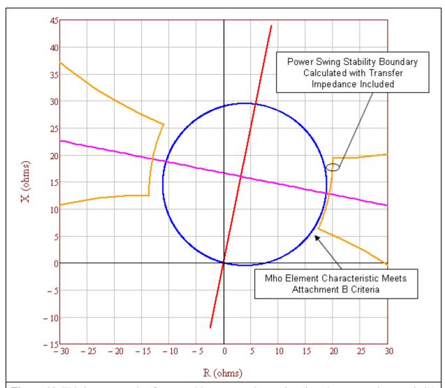
**Figure 11.** This is an example of an unstable power swing region (i.e., the orange characteristic) with the transfer impedance included. The mho element characteristic (i.e., the blue circle) meets the PRC-026-1 — Attachment B, Criteria A because it is completely contained within the unstable power swing region. However, including the transfer impedance in the calculation is not compliant with PRC-026-1 — Attachment B Criteria A.
