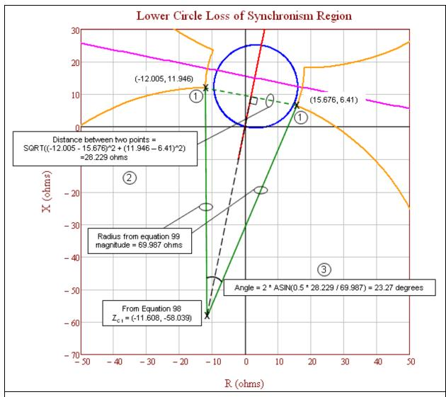
**Figure 15b:** Lower circle loss of synchronism region showing the first steps to calculate the coordinates of the points on the circle. 1) Identify the lower circle points that intersect the lens shape where the sending-end to receiving-end voltage ratio is 0.7 (see lens shape calculations in Tables 2-7). 2) Calculate the distance between the two lower circle points identified in Step 1. 3) Calculate the angle of arc that connects the two lower circle points identified in Step 1.
