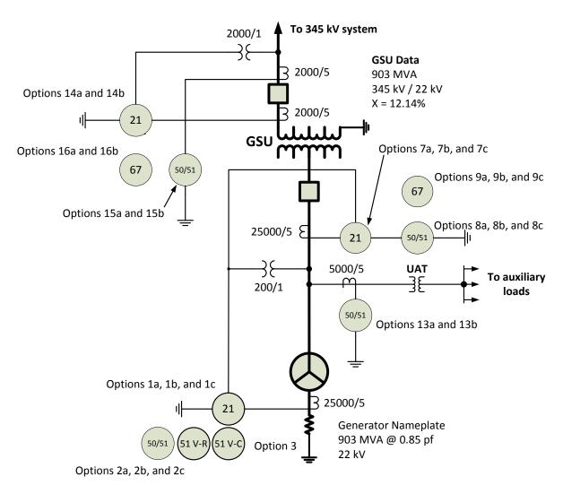
Figure 5: Relay Connection for corresponding synchronous options
