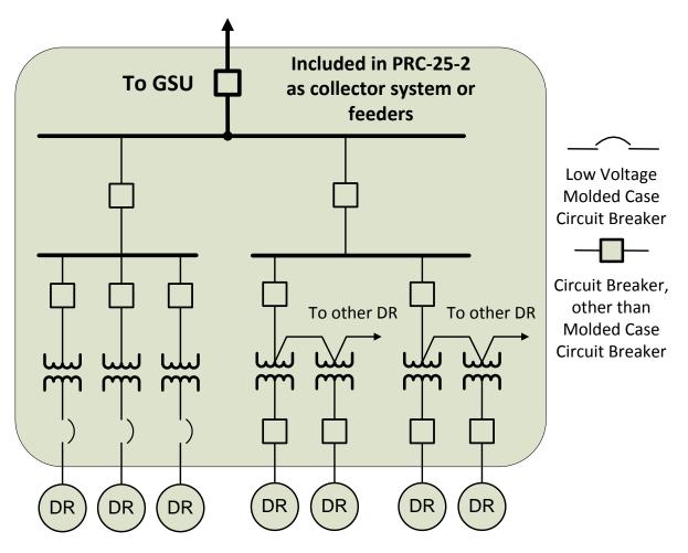
Figure-4: Elements utilized in the aggregation of dispersed power producing resources (DR)
