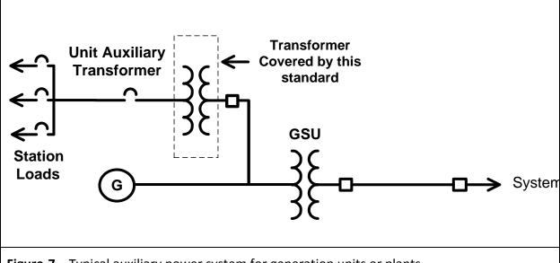
**Figure-7** – Typical auxiliary power system for generation units or plants.
