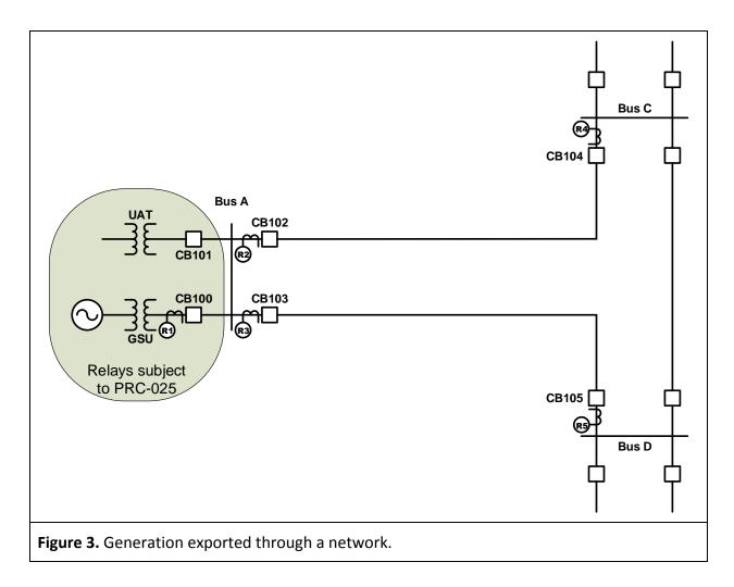
Elements utilized in the aggregation of dispersed power producing resources (in some cases referred to as a "collector system") consist of the Elements between individual generating units and the common point of interconnection to the Transmission system.
