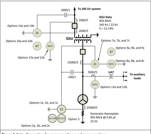
Figure 4. Relay Connection for corresponding synchronous options.
