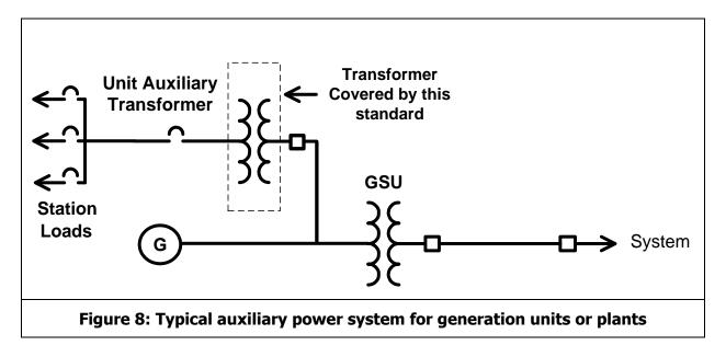
The UATs supplying power to the unit or plant electrical auxiliaries are sized to accommodate the maximum expected overall UAT load demand at the highest generator output. Although the transformer nameplate MVA size normally includes capacity for future loads as well as capacity
