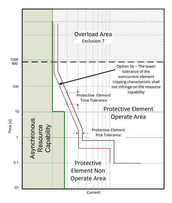
**Figure A**This figure is for demonstration of Option 5b and does not mandate a specific type of protective curve or device manufacturer.
