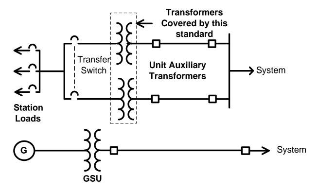
Figure 7: Auxiliary Power System (independent from generator)
