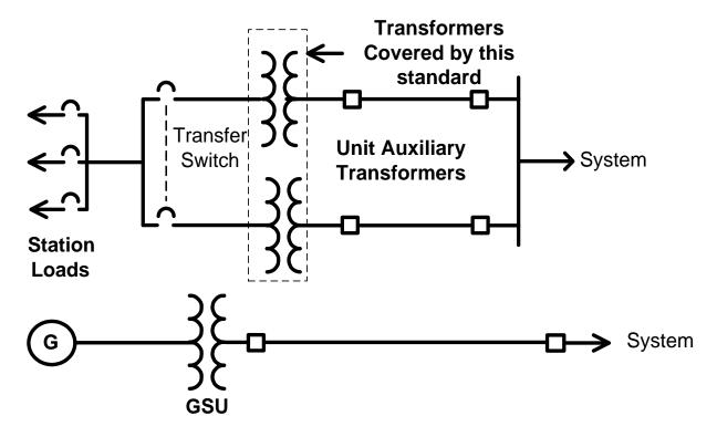
Figure-6-7: Auxiliary Power System (independent from generator).
