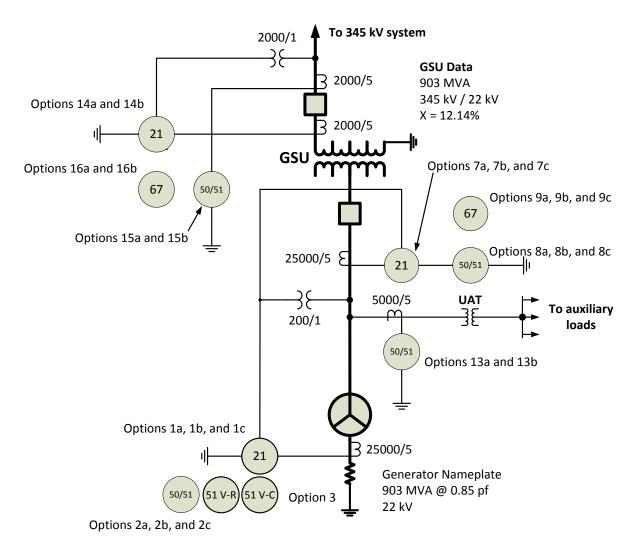
Figure 4.5: Relay Connection for corresponding synchronous options.
