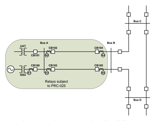
Figure 2-: Generation exported through multiple radial lines-
