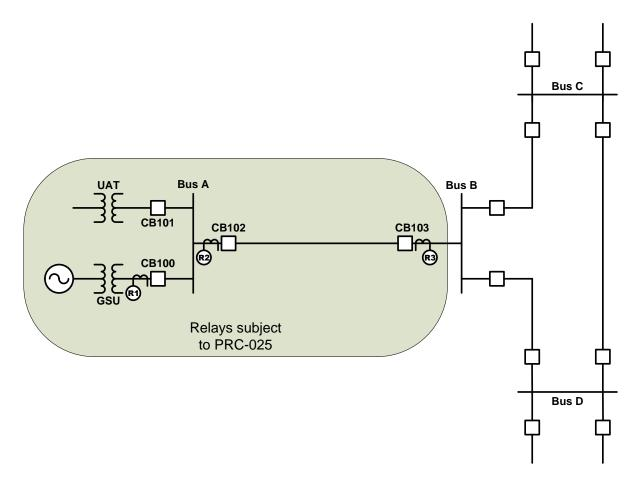
Figure 1-: Generation exported through a single radial line-
