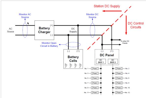
Figure 5–12 — Station DC Supply and Monitoring
