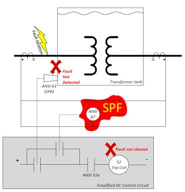
Figure 2.2: External Transformer Tank Fault with Sudden Pressure Protection and failed Transformer Differential Relay
